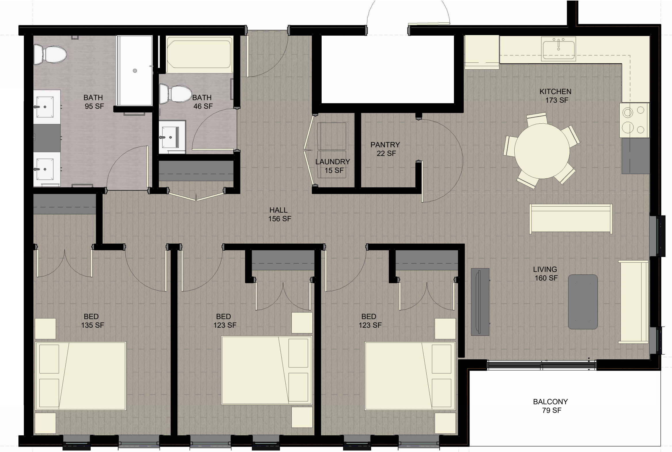
FLOOR PLAN - 3 BED / 2.0 BATH at BLDG SE CORNERS - TYPE B 1,160 SQUARE FEET
